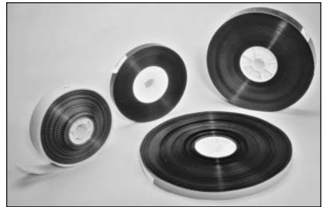
The edge of a poorly wound film is uneven and extends above the flat surface of the roll.
