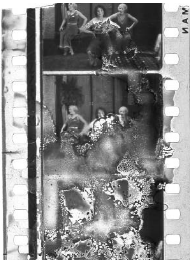
Nitrate “blooms” on a film in stage-two nitrate decay.
